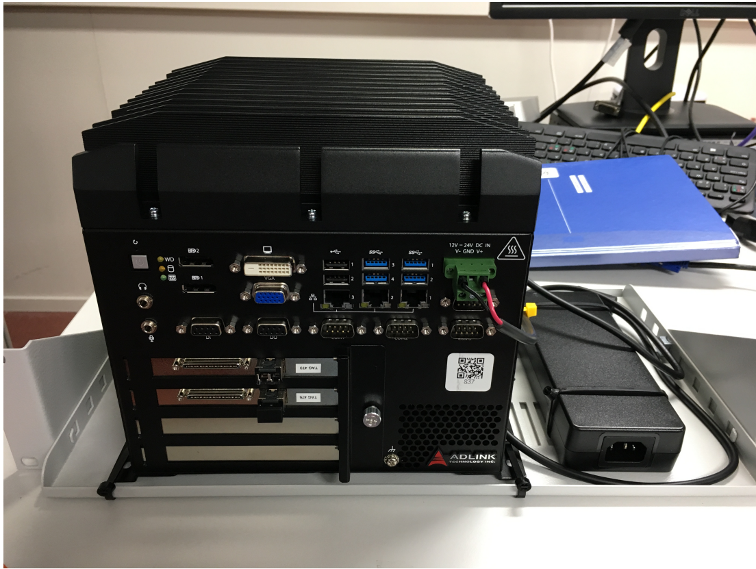
Figure 1 Hardware put together ready for rack installation. The cable from the PCIe-EVR-300DC to the IFB-300 should be connected with the system powered down.
