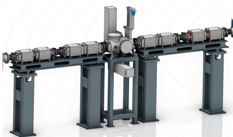
Figure 1: A drawing of how the full ESS raster system could be built, featuring 8 raster magnets in total. It should be noted that the central diagnostics chamber and support are not part of the package.
