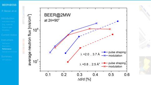
Dashed line shows the extension of the resolution range by adding the 3<sup>rd</sup> chopper as suggested for the staging plan.
