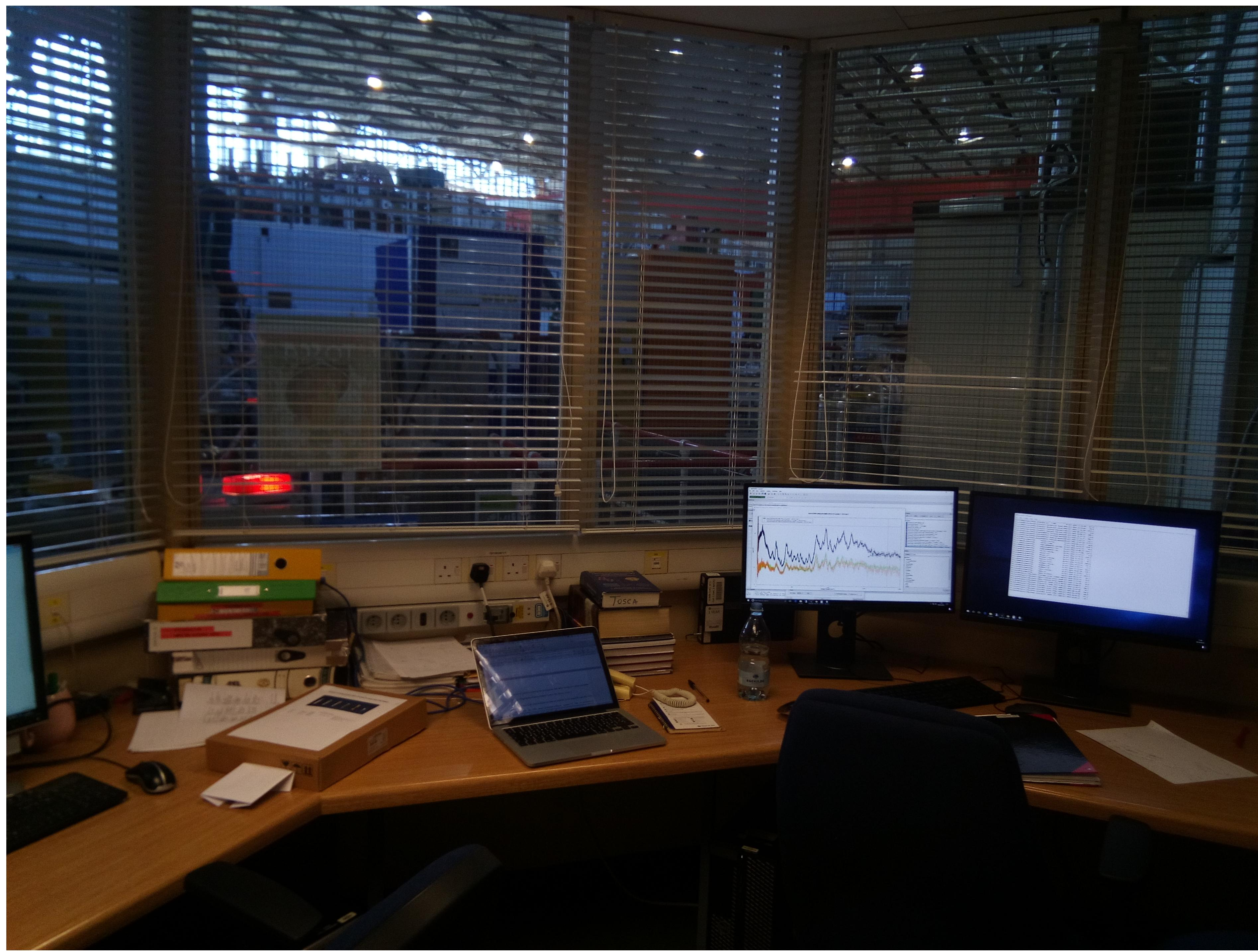
the TOSCA team (ISIS, RAL, UK) kindly provided me with a picture taken in the their cabin: the PC screen shows the MANTID software which is used for the data reduction from time-of-flight raw histograms to energy transfer spectra.
