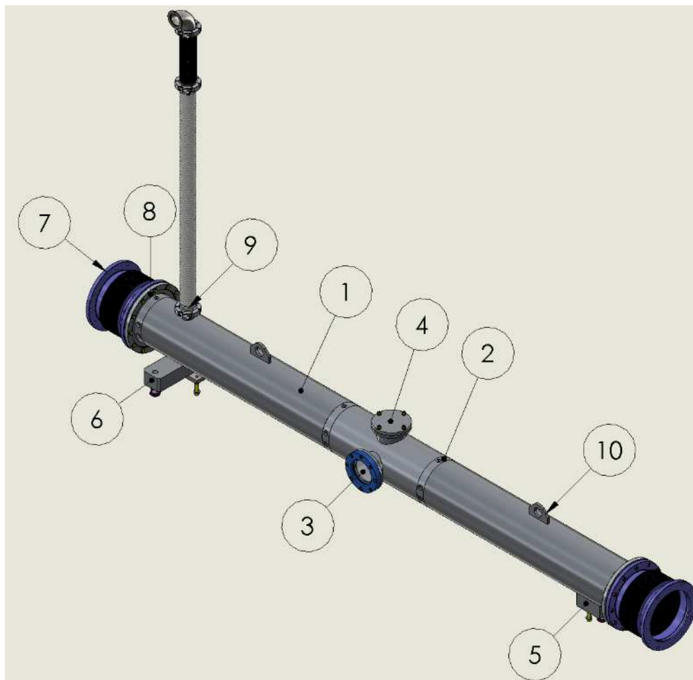
Figure 44: Overview of the fourth vacuum housing.
