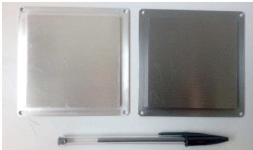
Figure 7 : Slow module cathode, without (left) and with (right) a 1.5 \mu\text{m} B 4 C neutron convertor layer deposit done at the ESS Detector Coatings Workshop, Linkoping.
