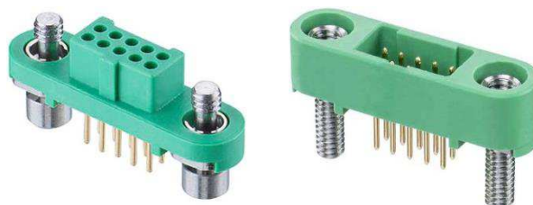
Figure 4: Harwin Gecko Screw-Lok Vertical DIL PC Tail Connector, with reference G125-MV11005M2P and G125-FV11005F1P (more info in HARWIN webpage or in document [5]).
