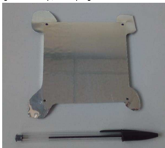
Figure 8 : Fast module cathode, with a 100 \mu\text{m} Mylar aluminized layer for neutron conversion.
