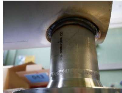
Outer vessel welding
