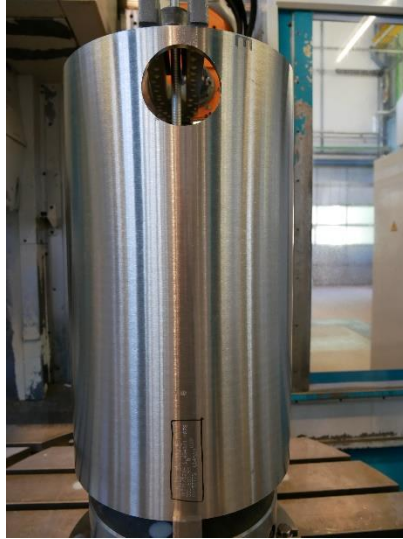
Outer vessel milling
