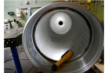
Inspection of inner welds
