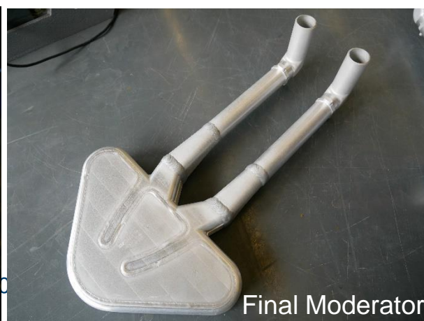
TIG welding of transition pipes
