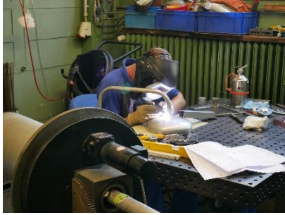
Welding of formed head
