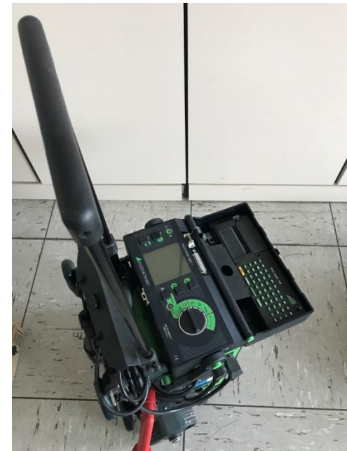
Metra machine (2kV)
