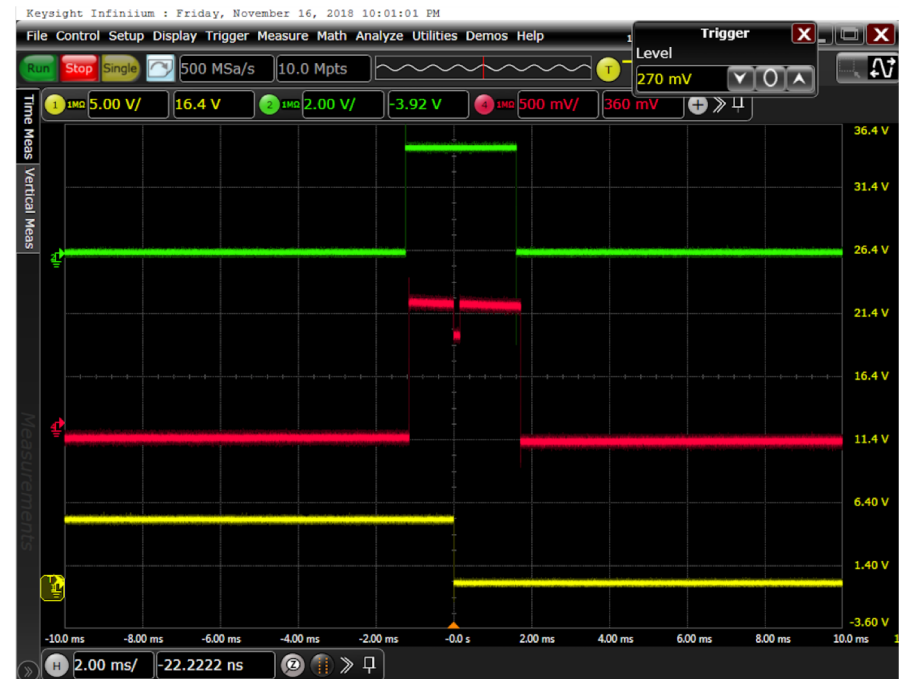
Interlock on too-low beam
