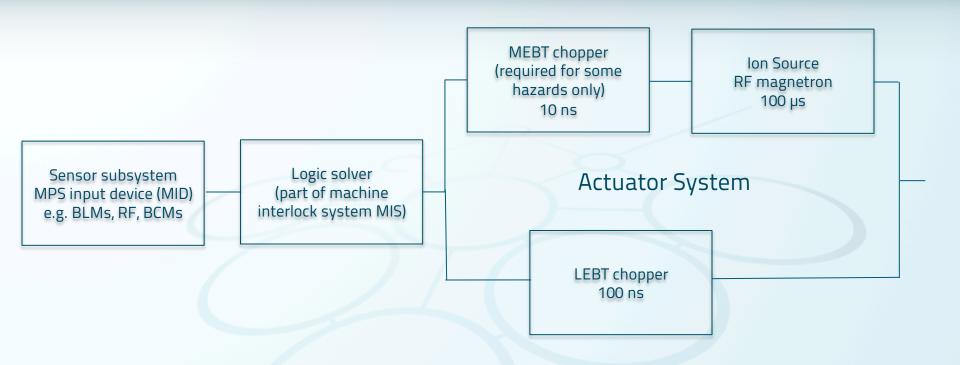
Two different mitigation techniques will be implemented Intra-pulse (within a pulse): fast beam stop Inter-pulse (in between pulses): let the current pulse pass (safe beam parameters) BUT inhibit the next *n* pulses
