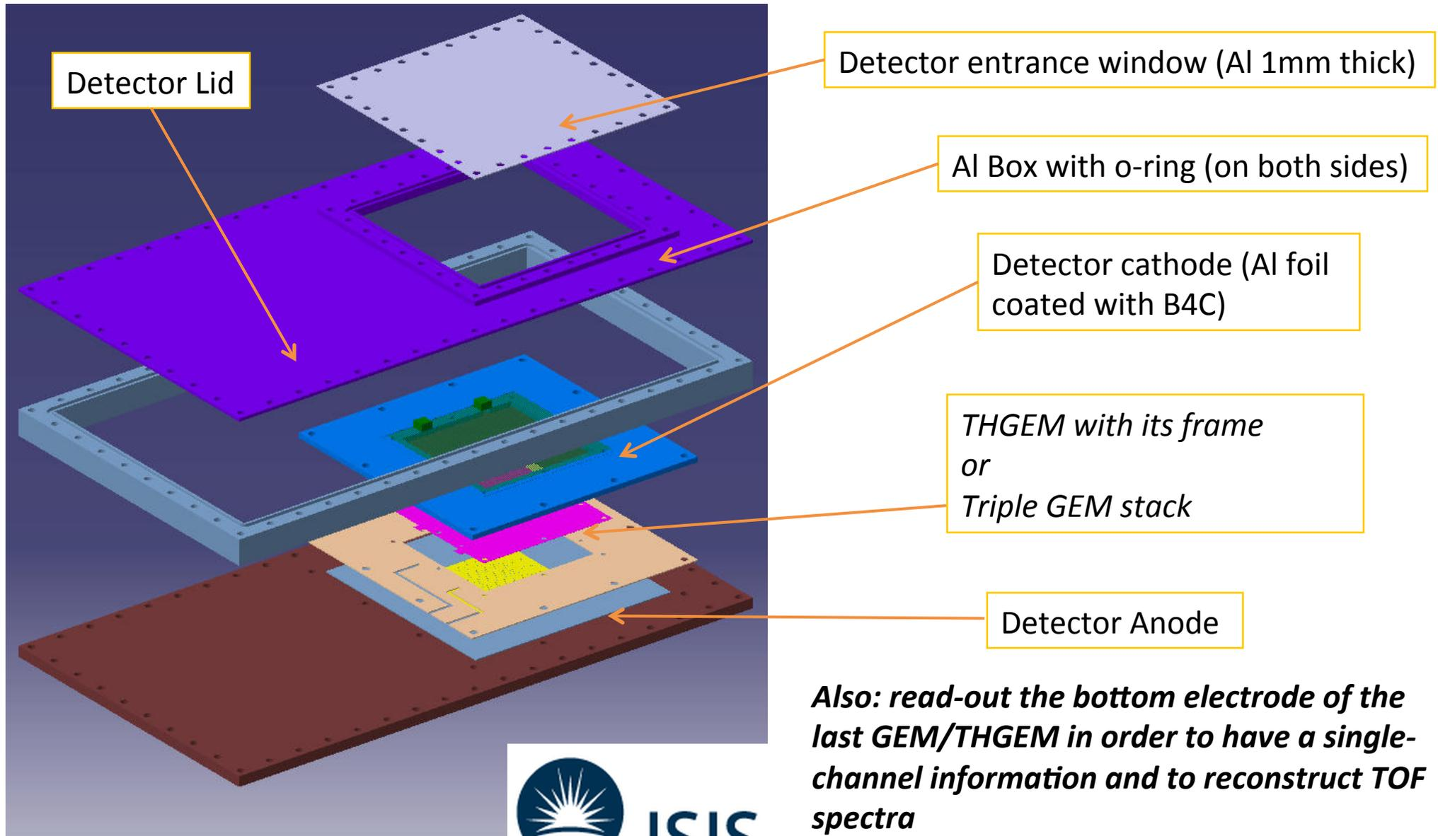
***Also: read-out the bottom electrode of the last GEM/THGEM in order to have a single-channel information and to reconstruct TOF spectra***
