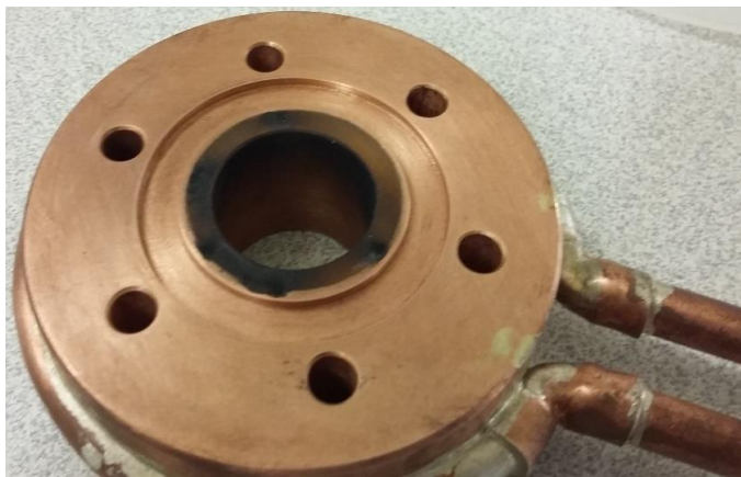
(c) A small water-cooled collimator aperture has been installed during the second campaign.
