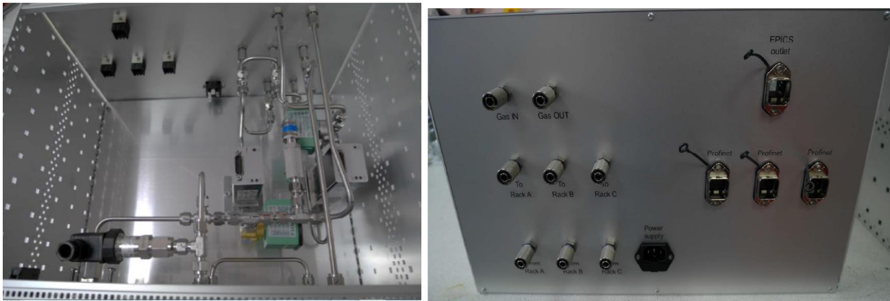
Figure 8: Inner view (left) of the main gas rack chassis. (Right) View of the back panel with the electrical connections and output of the distribution gas lines.
