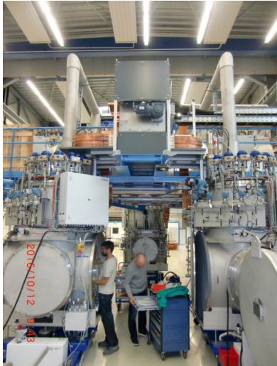
Electrical switch for 14 kA between 2 benches The 4. bench operated mainly for the serial testing of main current leads (MCLs)
