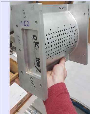
1 prototype passed the hydrostatic test.
