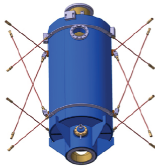
Figure 4.120: Helium vessel with hanging rod
