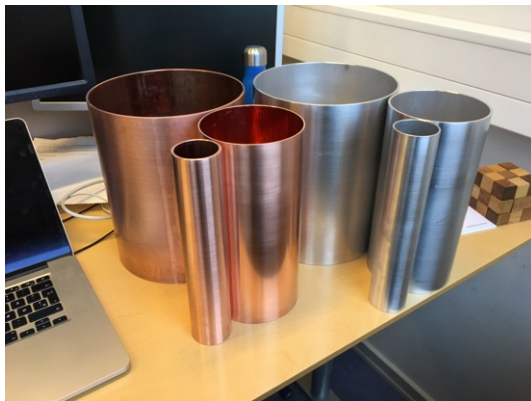
Figure: left: "Fake" sample environment for the verification of multiple scattering simulations. right: Copper cylinder in position on V20
