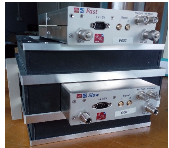
Assembly of a fast and a slow detector size \approx 20 \times 25 \times 25 \text{ cm}^3 ( \sim 14 \text{ kg} )
