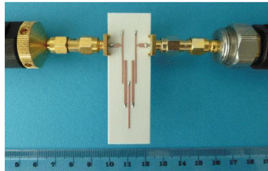
Ultra Wide Band filter for 2000 MHz, bandwidth 600 MHz (39%)
