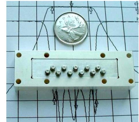
Waveguide filter for 22 GHz, size 50x13x10 mm, designed for MWTG, Canada
