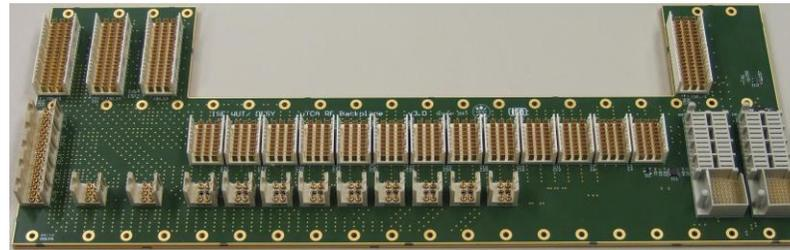
**Automatic test stand for MTCA.4 RTM
