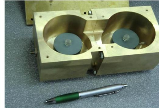
High quality filter for 1300 MHz, bandwidth 360 kHz (0.028%), IL=1.5 dB, thermal stability 2 ppm/°C, designed for DESY, Germany
