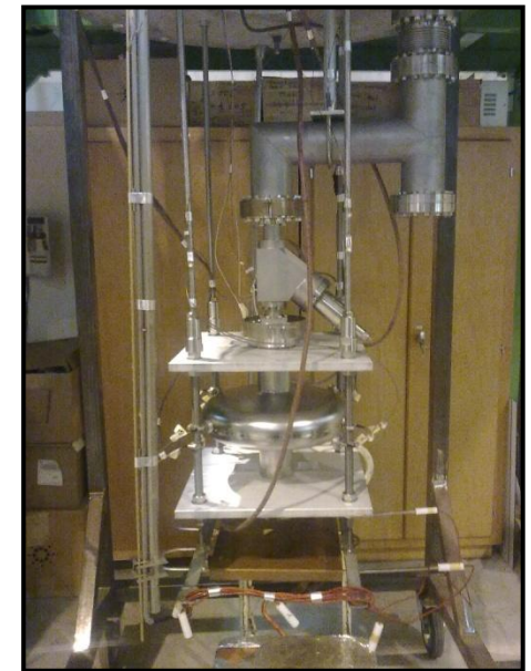
SPL mono-cell ( \beta=0.6 ) ready for vertical test - Courtesy of Mathieu Therasse
