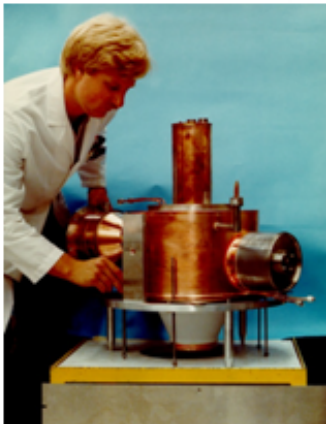
SDI, Integral Cavity 425 MHz 500 kW pk., 70% \eta
