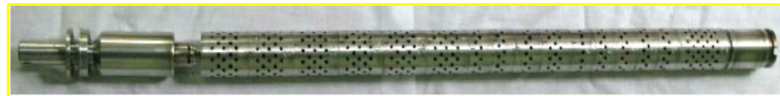
Assembled Suspension with 16 sample/monitor holders
