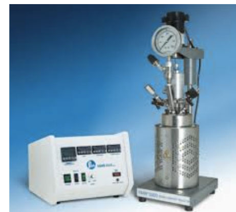
A Parr reactor for high-temperature, high-pressure chemical synthesis
