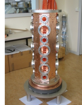
Design exists for ESS RFQ similar to 5 m long IPHI RFQ at Saclay. Energy 75 keV \rightarrow 3.6 MeV.
