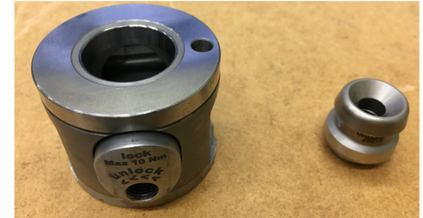
Kipp components: instrument part (left) equipment part (right). Each interface consists of three pairs
