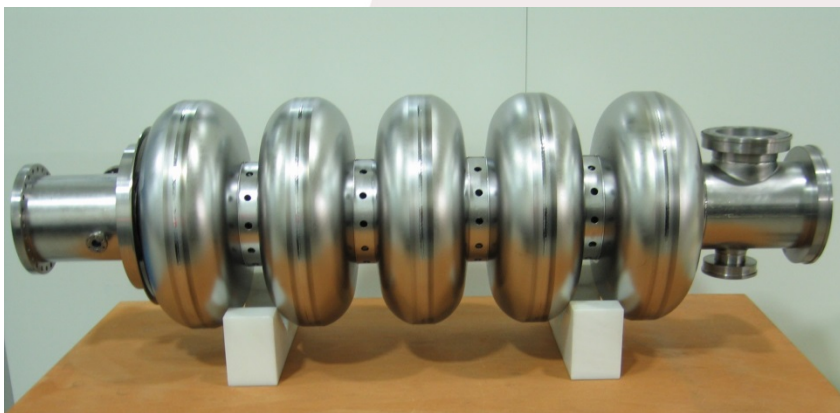
1 st high beta prototype cavity 5-cells – \beta=0,87 Before He tank welding
