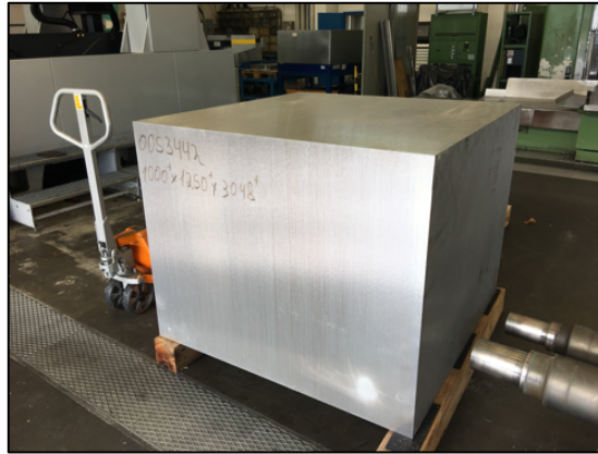
Figure 1. Al proto-material for the sample vessel inside FZJ workshop.
