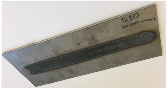
Steel to aluminum Friction melt bonding joint
