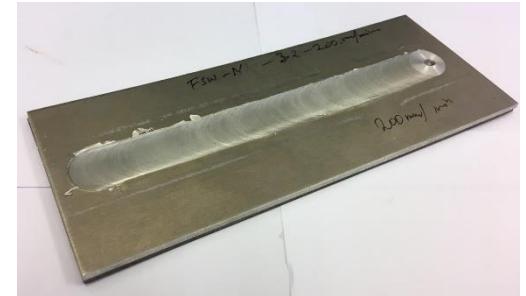
Steel to aluminum Friction stir weld
