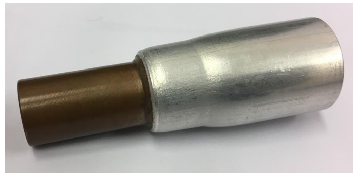
Copper to aluminum Magnetic pulse weld
