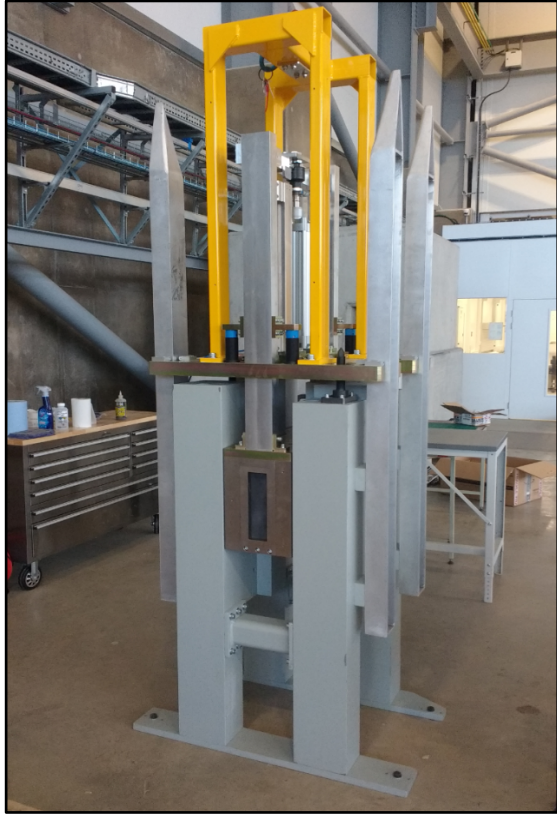
LoKI Heavy Shutter assembled at ISIS and ready for testing
