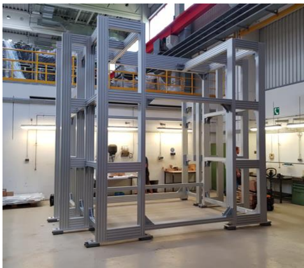
Fig.1. Detector support structure installed in FZJ
