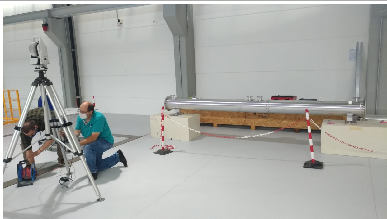
Figure 2: 4 m long guide housing ready for alignment and deformation checks.
