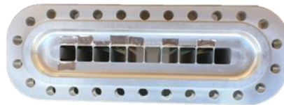
MultiTube beam monitor with the coated foils in place.
