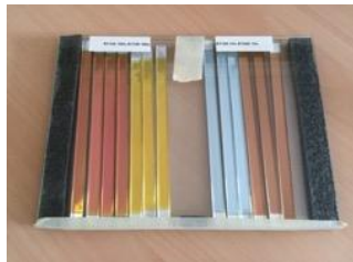
Thin Al foils coated with various B 4 C thicknesses. They are folded and fixed inside the MultiTube monitor cells.
