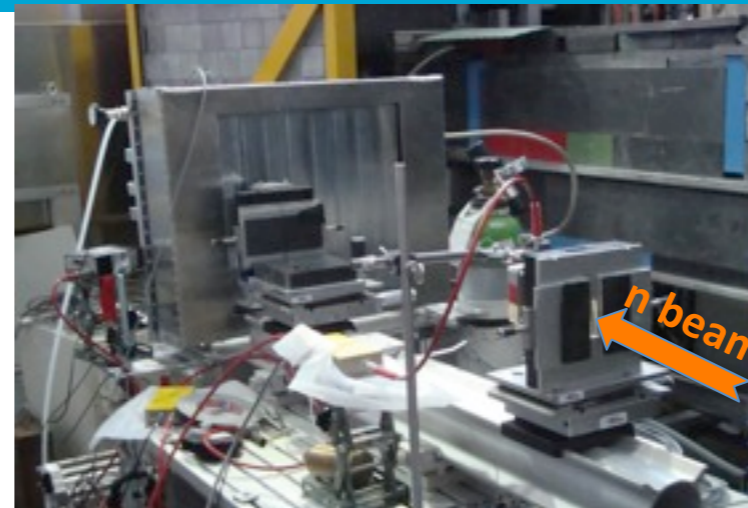
Photograph of the ^{10}\text{B} -demonstrator during the in beam tests at TREFF@FRM2 ( \lambda = 4.7 \text{ \AA} ).
