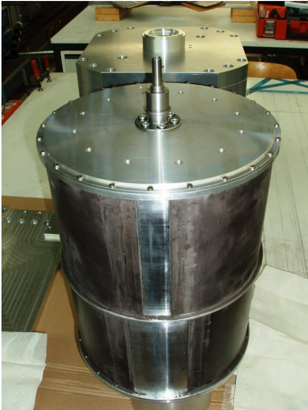
Low Speed Fermi Chopper (6000 rpm) with absorber coated (inside/outside) rotor MARIA, FRMII
