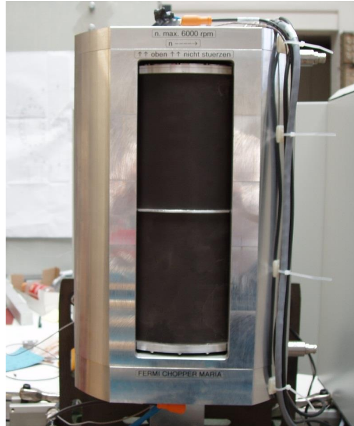
Low Speed Fermi Chopper (6000 rpm) with absorber coated (inside/outside) rotor MARIA, FRMII
