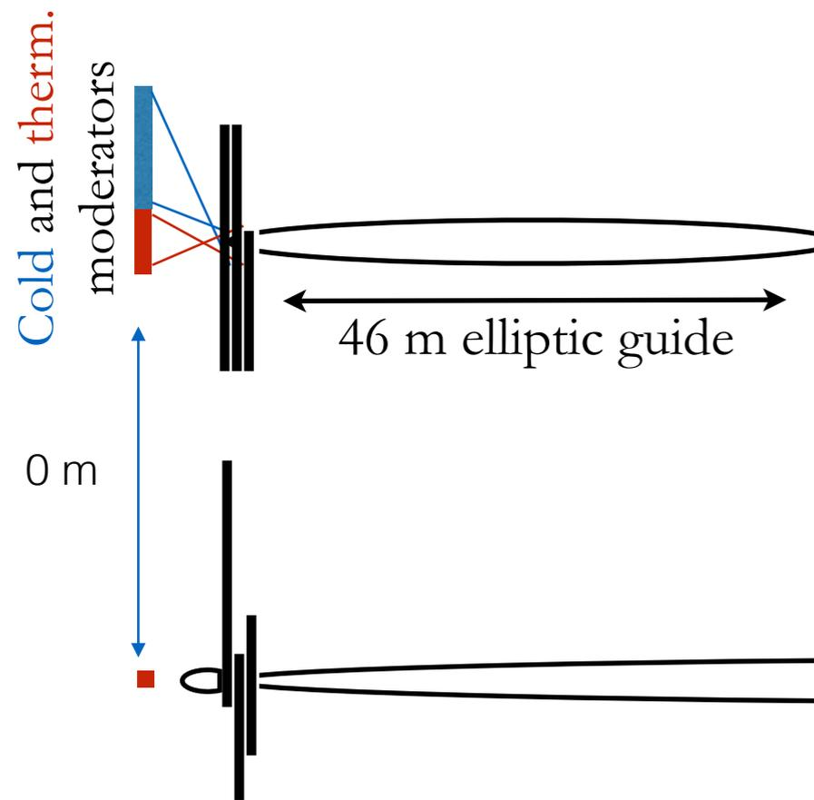
1st elliptical section: FeSi coated (left/right) and NiTi coated (top/bottom)
