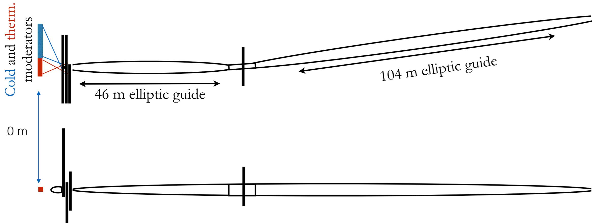
2<sup>nd</sup> elliptical section: FeSi coated (left/right) and NiTi coated (top/bottom)
