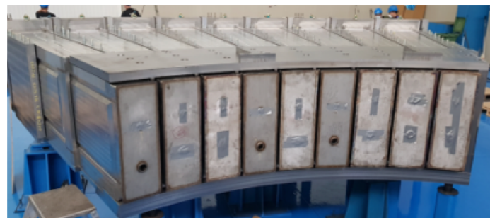
Proton Beam Window Vessel and port block parts ready to ship to ESS
