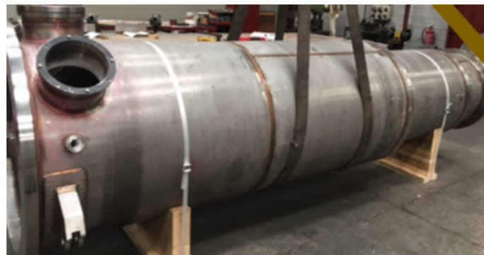
Proton Beam Window Vessel and port block parts ready to ship to ESS
