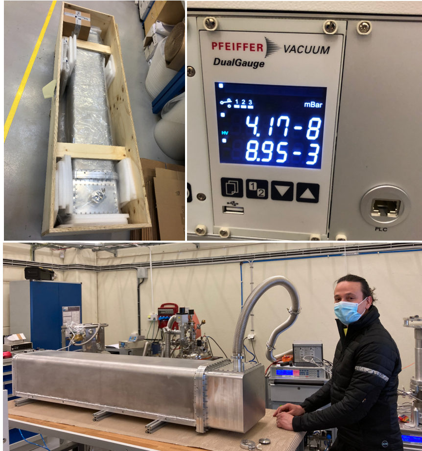
Figure 3 MG.CSPEC-BDO as it arrived at Utgard (top left). Vacuum reading after 1 hour of pumping down (top right). Alessio Laloni setting up the vessel for the vacuum test (bottom)
