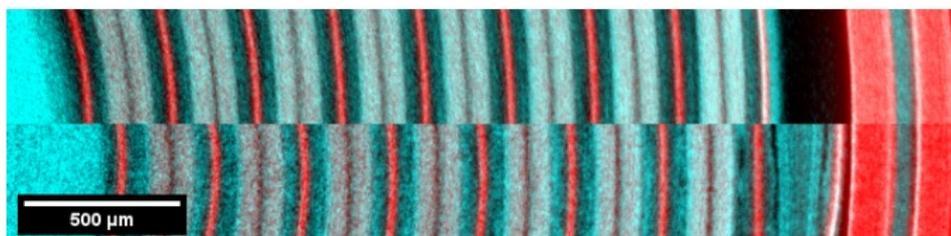
Figure 1. Cropped horizontal slices of Li-ion battery coin cells. Pixel size is 4.2  $\mu\text{m}$ . Combined NCT (cyan) and XCT datasets (red). Comparison of an unaged reference cell (top) with a highly cycled cell (bottom).
