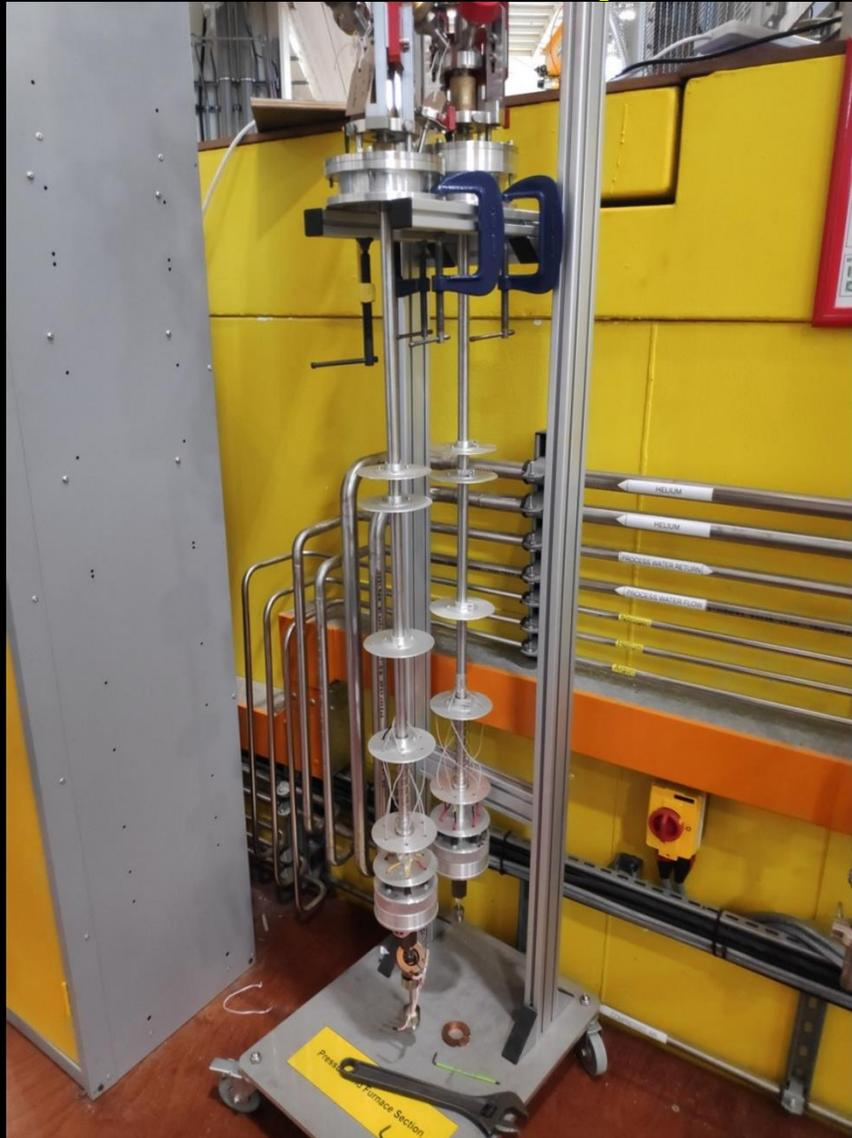
The stick is connected to the gas handling apparatus and to the high-pressure cell
