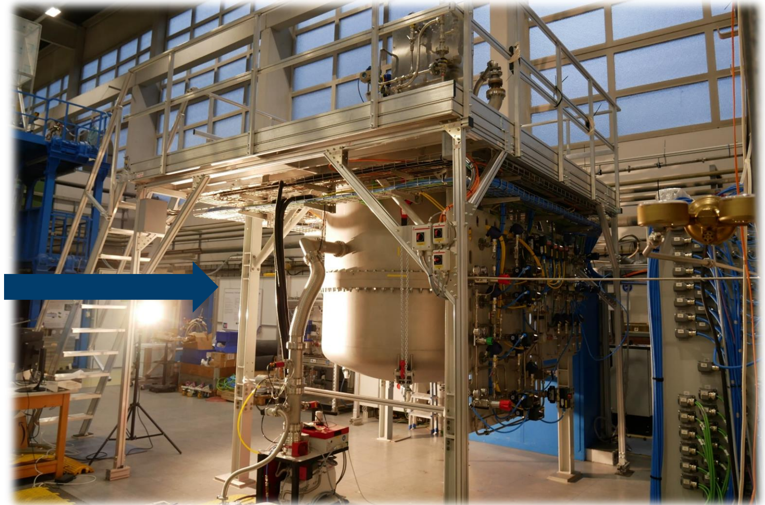
Hydrogen cryostat 5x5x4m; up to 1000 g/s LH2 @ 20 K and 10 bar
