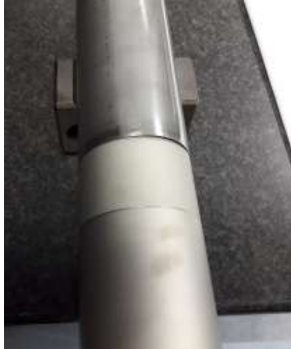
1 m prototype replica tube with ^{10}\text{B} foil inserted into cryostat mockup
