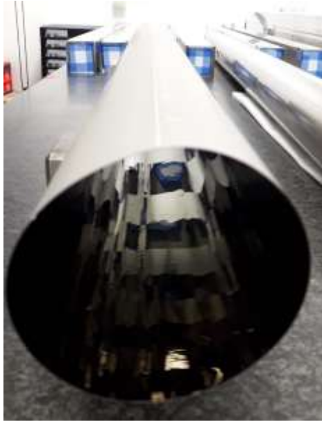
1 m prototype replica tube after welding
