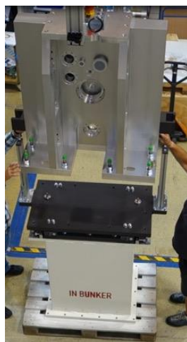
Figure 2 Left: remote handling test of band-control chopper housing; right: remote handling rails for the pulse-shaping chopper.
