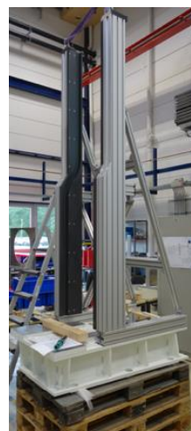
Figure 2 Left: remote handling test of band-control chopper housing; right: remote handling rails for the pulse-shaping chopper.
