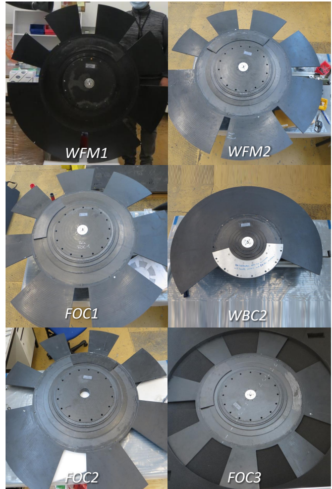
Figure 2 The 6 assembled carbon-fibre chopper discs for FREIA
