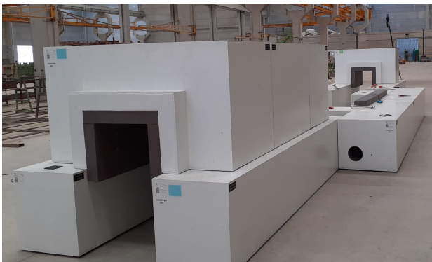
Figure 3. Shielding blocks of the chopper pit assembled during a test
