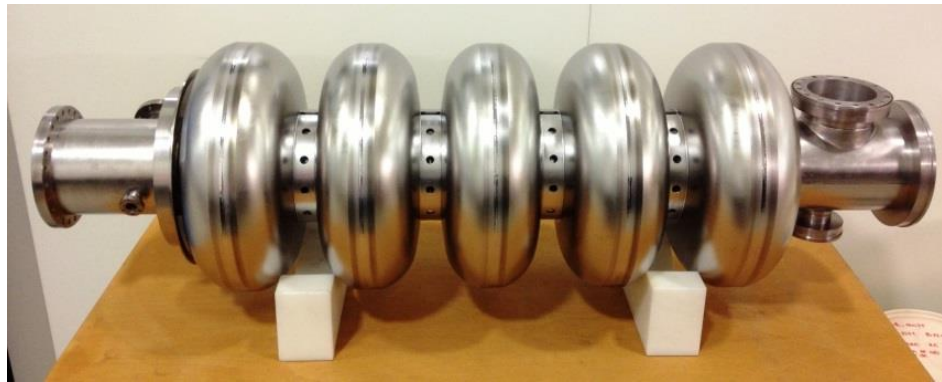
P01 manufactured by E. ZANON F_{\pi} = 703.553 MHz Field flatness: 86%
