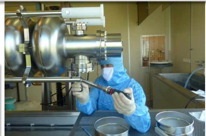
Flanges and antenna pick-up assembly under class 100 laminar flow
