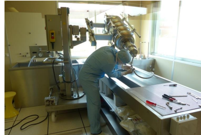
Flanges and antenna pick-up assembly under class 100 laminar flow
