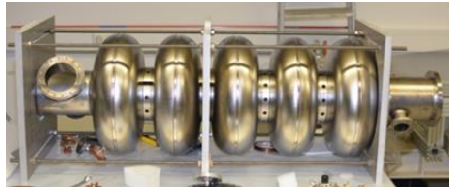
P02 manufactured by RI F_{\pi} = 703.704 MHz Field flatness: 40% Bad angles stiffning rings
