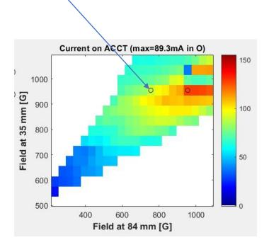
**PS-ESS** commissioning shows experimental physics correlation between magnetic field configurations and source behaviours
