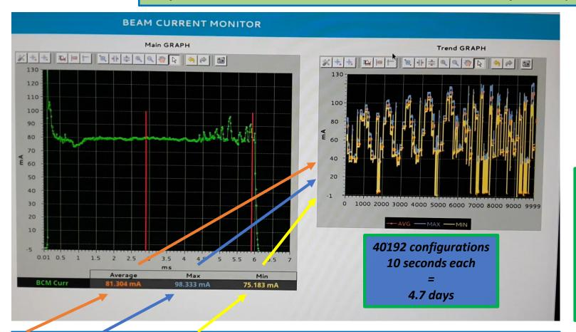
In the graphical interface: average, maximum and minimum are evaluated, and the trend showed for the beam pulse between 2.9 ms and 5.9 ms.
