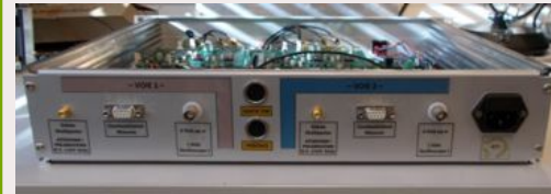
Electronics boards for power coupler conditioning
