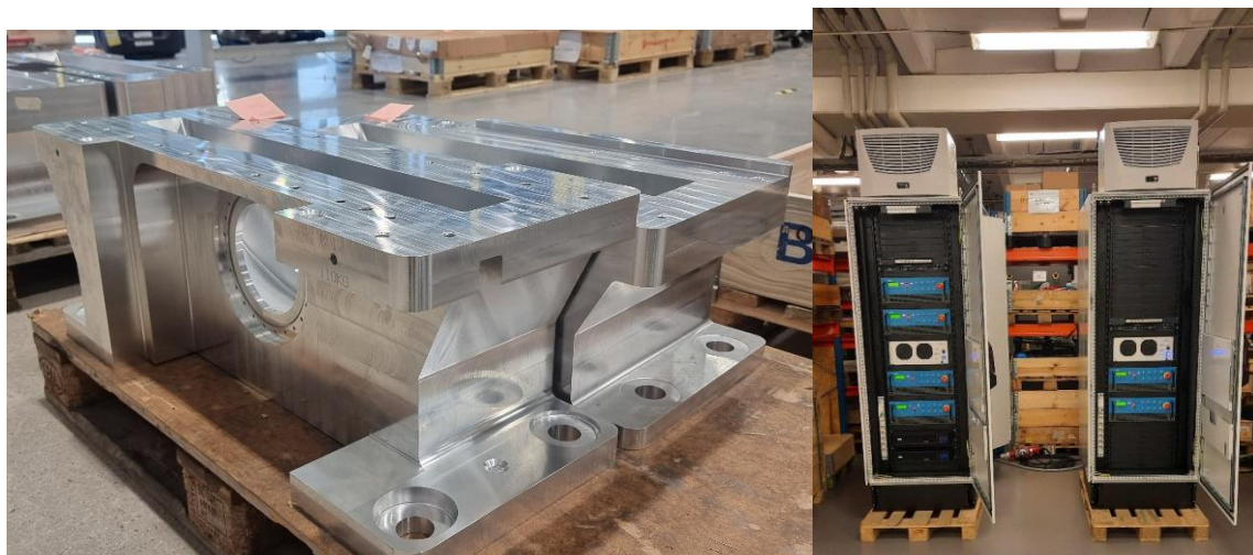
Figure 2: (left) Chopper housings for BIFROST. (right) Chopper control racks
