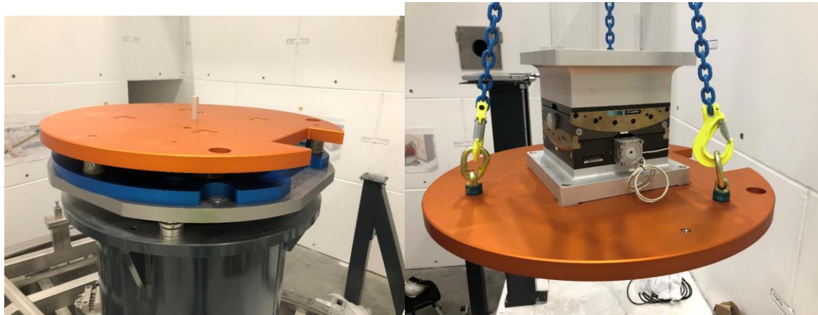
Figure 4:(Left) Sample stack assembly. (Right) Orange cryostat base including goniometer
