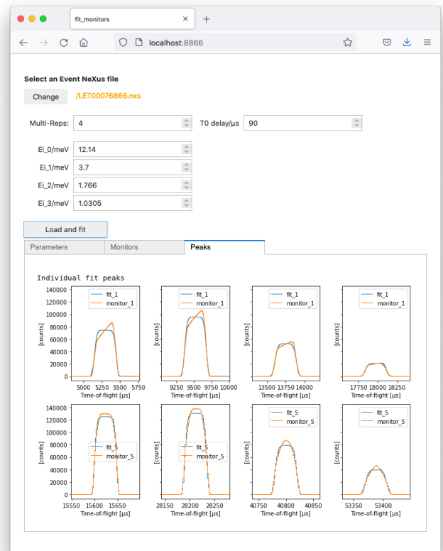
Figure 7: The Jupyter notebook based Voila GUI: monitor spectra and fit peaks in the regions surrounding the monochromatic energies.
