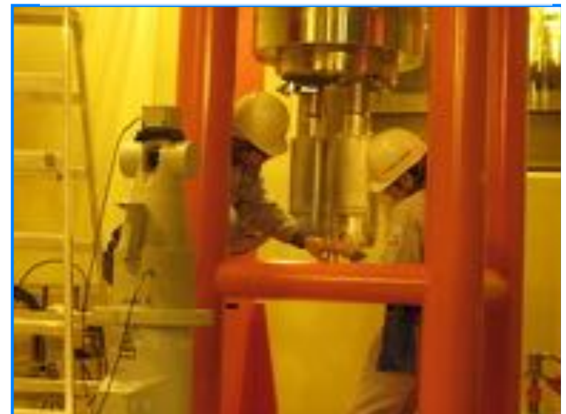
Moderator position was surveyed very precisely by a laser tracker.
